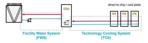
**Water** is a very effective heat transfer medium. Its electrical conductivity restricts its use to cold plate technologies, where it does not come into direct contact with the electronic components it is cooling. It is also used by many immersive solutions within TCS loop and FWS loop.
